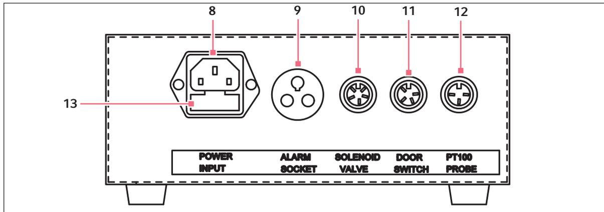
Fig. 3-2: Back view of the CO<sub>2</sub> Back-up System
