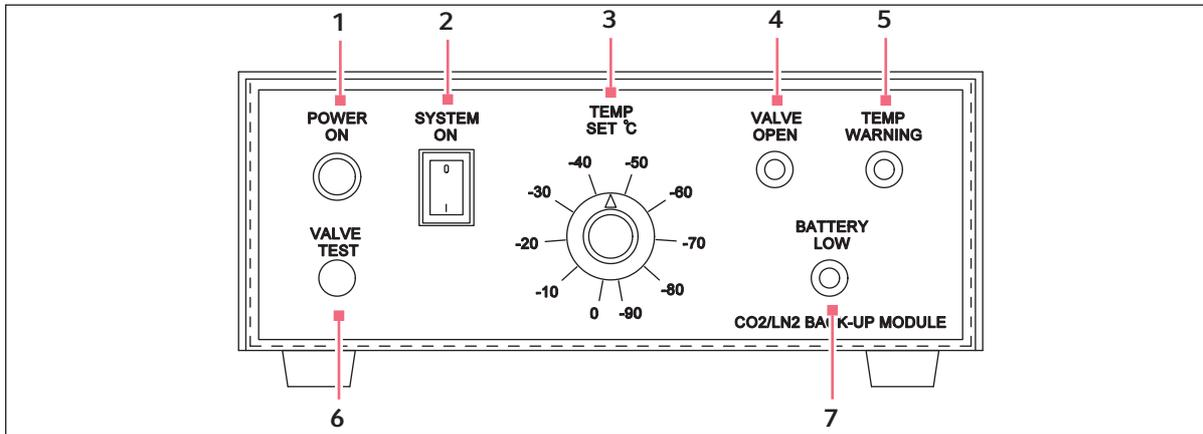
Fig. 3-1: Front view of the CO<sub>2</sub> Back-up System
