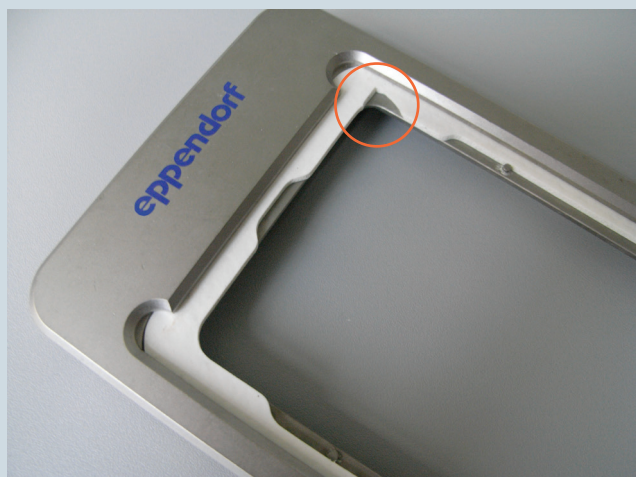
Figure 3: Vac frame 2 with nicked silicon insert
